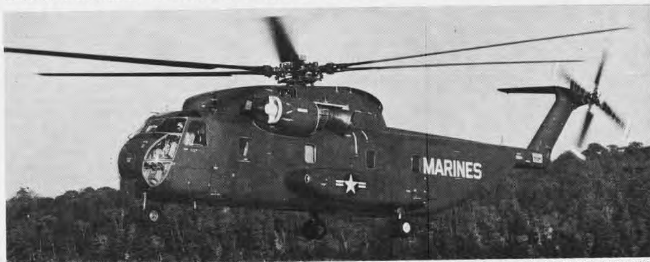
MARINE'S NEW HEAVY ASSAULT HELICOPTER IS THE SIKORSKY CH-53A. FIRST FLIGHTS WERE MADE TO TEST HOVERING CAPABILITY
