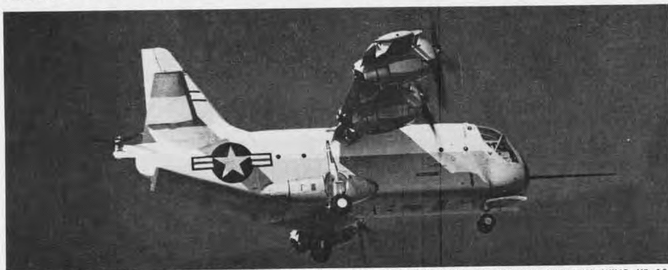
TRI-SERVICE V/STOL ASSAULT TRANSPORT, LTV-VOUGHT'S XC-142A, MADE THE FIRST FLIGHT AS AIRPLANE WITH TILT WING UP 10°
