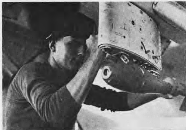
AN ORDNANCEMAN from VMA-531 secures a practice bomb on a squadron A-4E Skyhawk. The Marine wears a distinctive red jersey.
