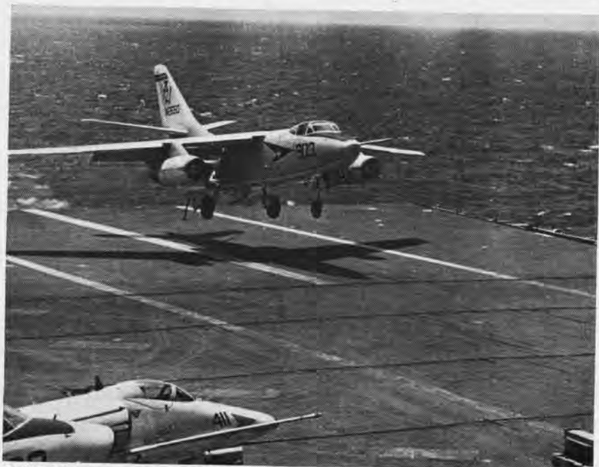
TAILHOOK DOWN , a Skywarrior returns home to the Forrestal . Cross-deck pendants are clearly visible as plane sets down. In a short while, "Secure from flight quarters" will be sounded.
