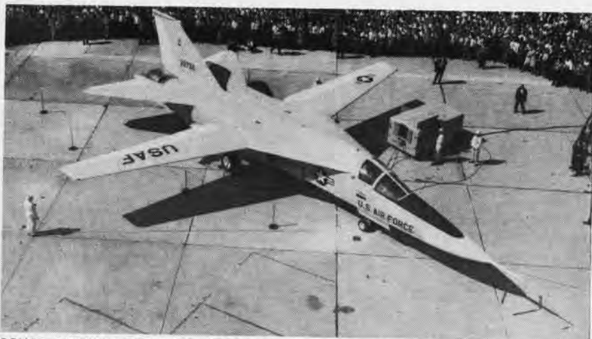
ROLLED OUT WAS FIRST F-111, SEEN HERE WITH WINGS FORWARD FOR SUBSONIC FLIGHT
