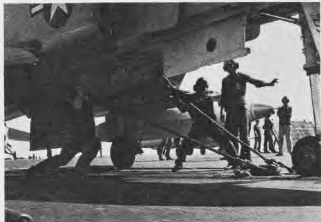
THE GREEN SHIRTS (the catapult workers) check the tension on the bridle of an F-4. In less than a minute, the plane will be launched.
