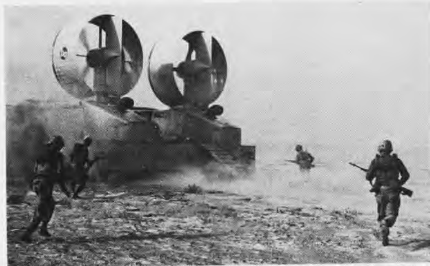
U.S. MARINES head for their amphibious air cushion vehicle (ACV), the 65-foot, 22½-ton Hydroskimmer after simulated raids on a beach near Buffalo, N.Y. The Marines were taking part in a test conducted by Textron's Bell Aerosystems Company for the Navy to determine the suitability of ACV's for various Navy missions. Still other tests are scheduled. The ACV, the largest and most powerful one in U.S., was built by Bell under a Bureau of Ships contract.
