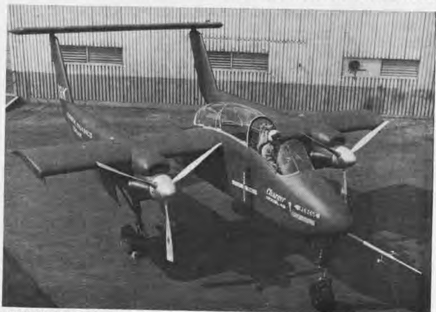
GD/CONVAIR'S 'CHARGER,' A COIN PROTOTYPE, HAS LAYOUT LIKE NAA'S COMING OV-10A
