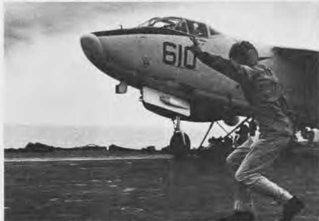
THE CATAPULT OFFICER gives the signal to go. The pilot in the A-3B braces for as many as 3.69 G's he can expect during the launching.
