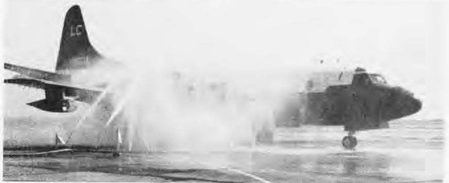
IT'S A THREE-MINUTE WASH for this Orion at NAS Patuxent River. This fast procedure is designed to help fight salt corrosion of low-flying ASW aircraft. It is a one-man operation, the five hydrant supplying the "wash" which can be turned on by a station line crewman on two or three minutes notice. Aircraft are completely rinsed from inside flap wells to the top of the tail by passing through the water one way and coming through again the other way.
