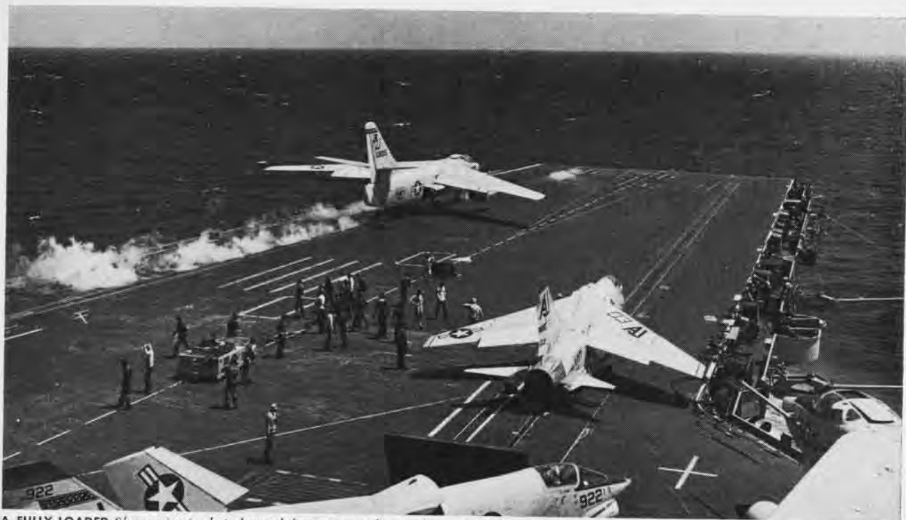
A FULLY-LOADED Skywarrior is shot skyward from Forrestal's number two catapult as an F-8C Crusader awaits its turn on the number one catapult. Most men here are wearing green shirts, though the yellow shirt of a plane director can be seen at the lower left side.
