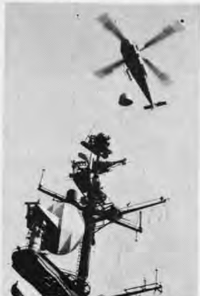
THREE MEN in FDR, perched at 185 feet and assisted by a helo, repair the ship's TACAN.
