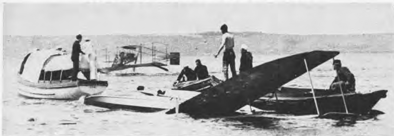
THE WRIGHT B-1 hydroaeroplane is salvaged after Herbster's 1912 crash in San Diego Bay, wing panel and floats in foreground. Evidence from repairs recently led surviving crewman to identify aircraft's engine, only major item still existing from Naval Aviation's beginning.
