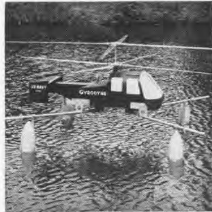
SCALE MODEL floats tilted to vertical position minimize motion in rough water state.
