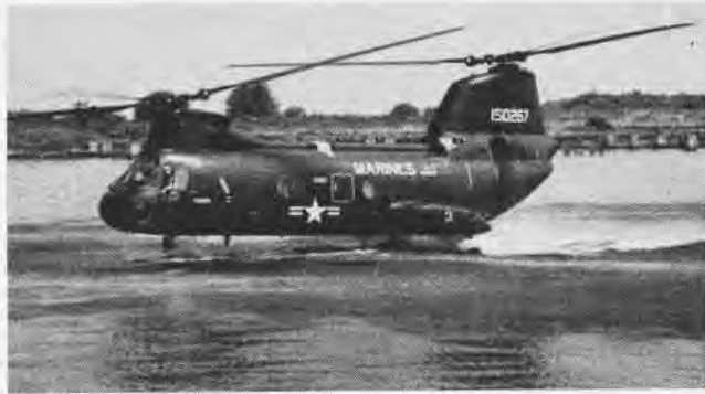
FROM THE HUP-2 , much was learned as is apparent to one studying the lines of the CH-46A. Fuel tanks provide the lateral stability needed.
