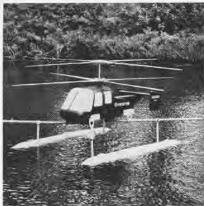
SCALE MODEL tilt-float helicopter rests in water with floats in normal flight position.
