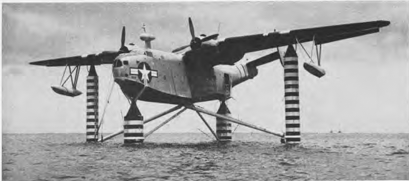
OLD PBM'S NEVER DIE. This bulk is completely instrumented to furnish information for design of a seaplane which can rest nearly motionless in the open ocean in all weather conditions. At the present time, it can be seen sitting out at sea off Point Loma, near San Diego, Calif.
