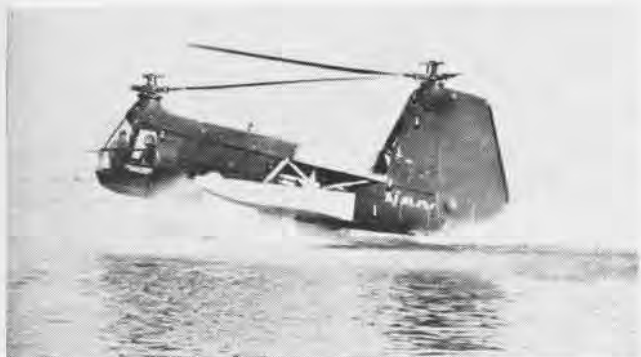
THE HUP-2 SEACOPTER was the first true amphibious helicopter to be planned and designed to meet rigid Navy seaplane specifications.
