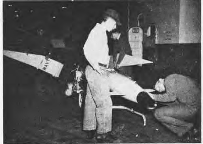
ON USS MIDWAY , men install the wings, fins, canards and nose section quickly by virtue of the simplicity of the design.
