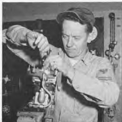
PUMP FOR CARGO DOOR IS REPAIRED
