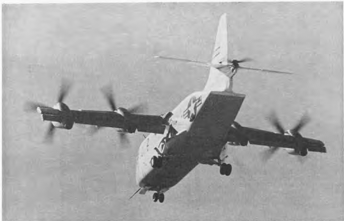
WITH WING APPROACHING DOWN POSITION, XC-142A ACCELERATES TOWARD CONVENTIONAL AIRPLANE FLIGHT AND FLIES AWAY
