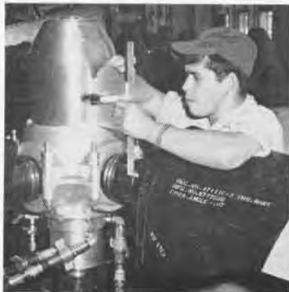
PROP IS CHECKED AS IF ON THE AIRCRAFT
