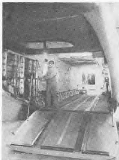
MOCKUP SHOWS cargo loading ramp and interior. Powered cargo-handling system is used.
