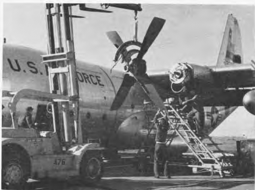
AT MOFFETT FIELD, MEN FROM POWER PLANTS DIVISION INSTALL A PROP ON C-130
