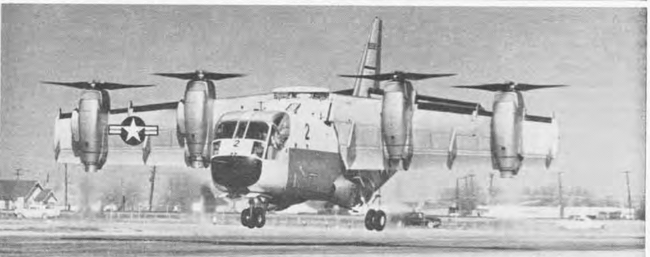
FROM HOVER, WITH PROPS CARRYING ALL 37,000+ POUNDS, WING IS TILTED FORWARD AND XC-142A STARTS INTO FORWARD FLIGHT
