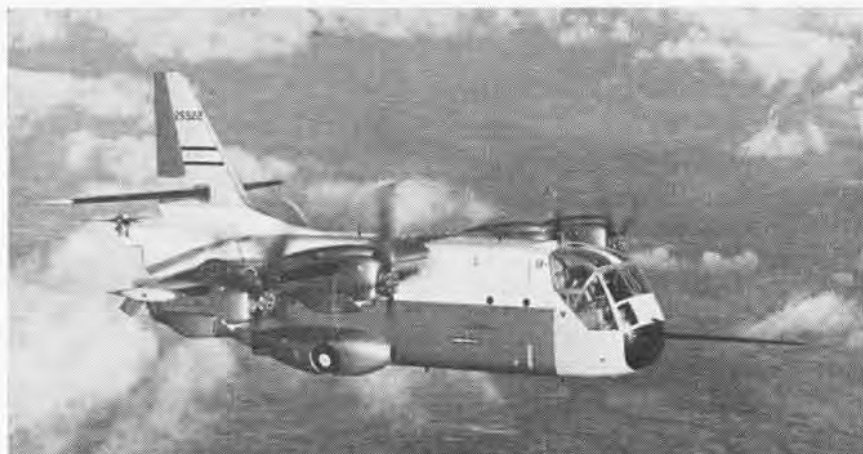
GEAR UP, WINGS DOWN, XC-142A REACHES SPEED OF CONVENTIONAL PROP PLANES
