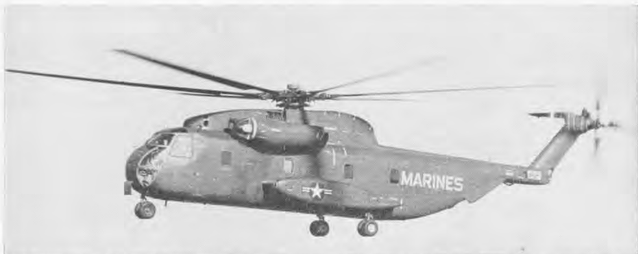
FIRST FLIGHT of Marine Corps' CH-53A took place over Sikorsky flight field in October 1964. Using only partial power, the new aircraft has been clocked at 200 mph. Manufacturing time and costs were reduced in many ways; for example, cockpit section is made of plastic.
