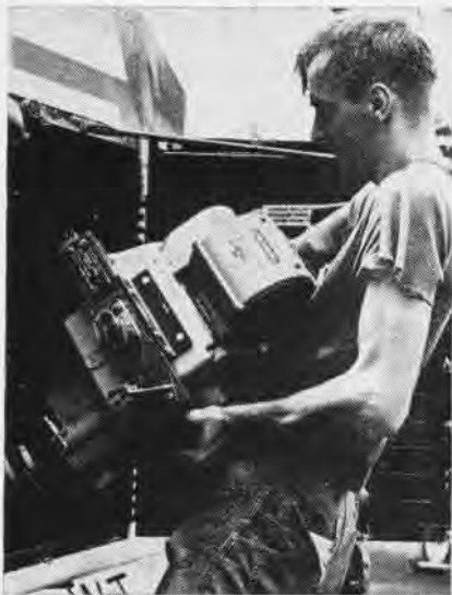
G. D. GILL, PH3, installs aerial camera in Crusader on flight deck just before launch.
