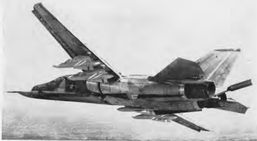
THE FIRST F-111 equipped with missiles under the wing has begun flight tests at Edwards AFB, Calif. Rotating pylons keep the externally carried weapons parallel to the fuselage during changes in the wing-sweep angle. The F-111 takes off with its wings set at a 16-degree angle, then sweeps them back to 72.5 degrees for supersonic flight. The rotating pylons automatically compensate for the changes in wing sweep.
