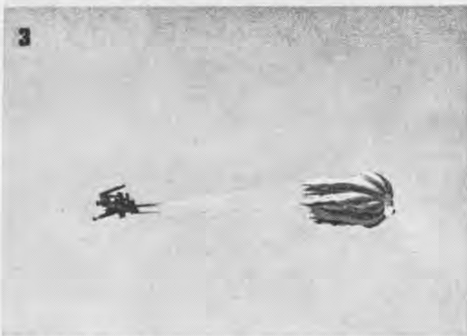
SUCCESSFUL FIRING of the new LW-38 escape seat system was accomplished at Holloman AF Base, New Mexico, in June. Developed by
