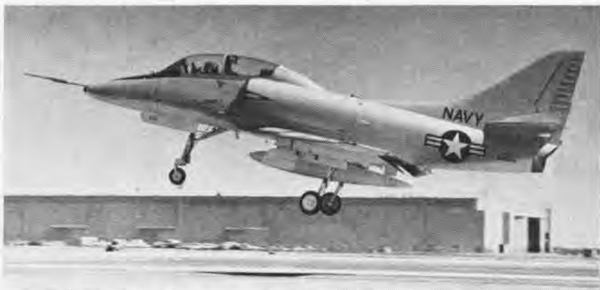
THE FIRST FLIGHT of the Douglas TA-4E Skyhawk took place on June 30 at Palmdale, Calif. The aircraft, featuring twin tandem cockpits, a zero-level ESCAPAC ejection system, a steerable nose wheel and wing spoilers, is programmed for delivery to the Fleet in April 1966. Powered by a Pratt & Whitney J-52-P-8A (the same power plant used in the A-6A), the advanced jet trainer can put out 9,300 pounds of thrust with a maximum speed of Mach 1. The initial order of 35 will be assigned to replacement training squadrons.
