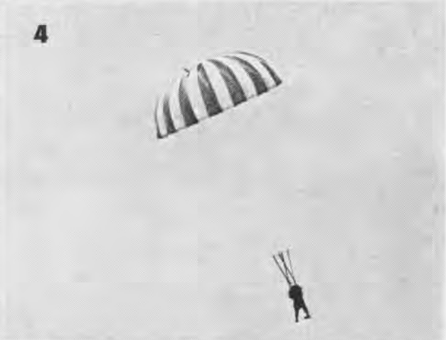
North American Aviation's Columbus Division for the OV-10A aircraft, the seat with a 210-pound dummy was ejected at 410 knots.
