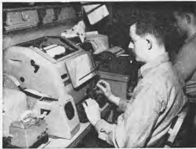
WORKING in Main Comm aboard Bon Homme Richard , L. E. Gunderson (L) operates ship's radio-teletype gear as L. A. Lawson types.
