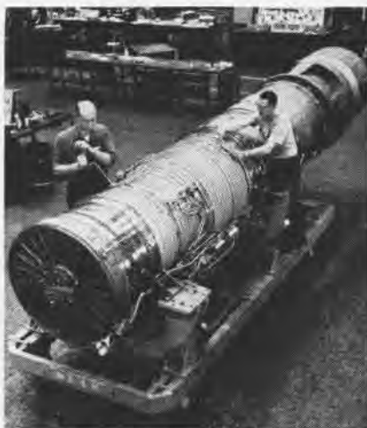
THE P&W TF 30P-1 turbofan engine, powerplant for the General Dynamics F-111 variable sweep wing fighter, has successfully completed official ground endurance tests required for military qualification, according to USAF. Grumman Aircraft is principal subcontractor for Navy version of the F-111.
