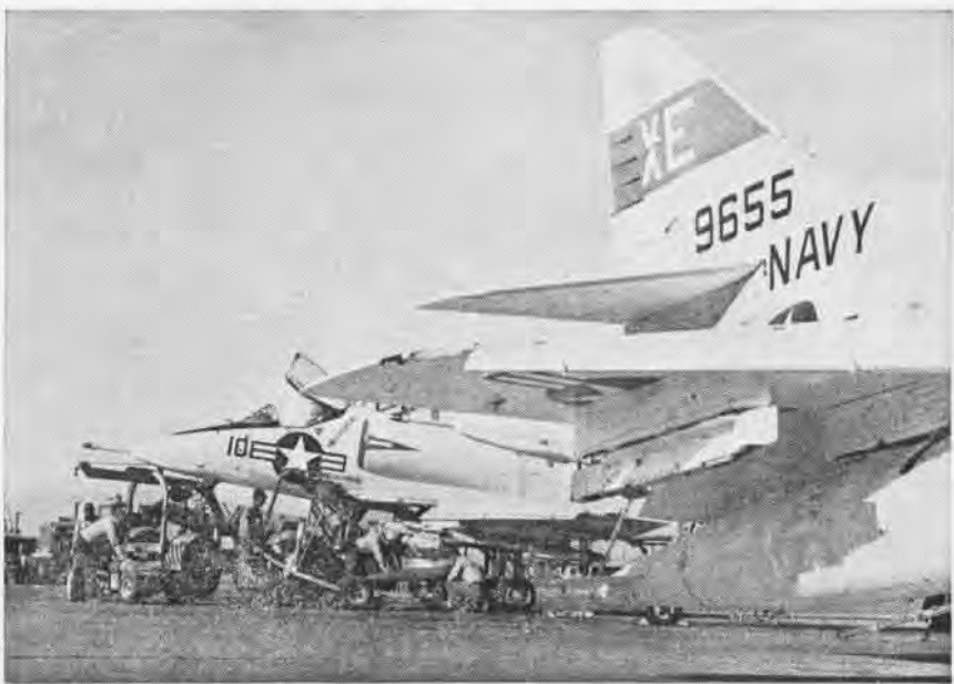
ON THE LOAD LINE , ordnancemen wheel up carts holding Mark 81 Snakeyes which are to be installed in the bomb racks. After the plane is loaded, the test flight will be made.
