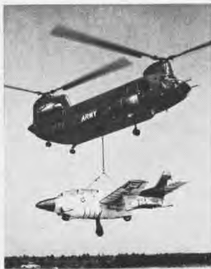
HEAVE-HO. The Army lends the Navy a helping hand as one of its CH-47A Chinook helos transports a T-2A Buckeye from NAAS Meridian to Overhaul and Repair, NAS Pensacola. The helo hoist of a 5,000-pound aircraft reduces the cost of dismantling the trainer and packing it for rail shipment.
