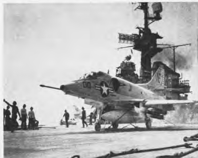
BOMB-LADEN A-4 Skyhawk assigned to VA-22 aboard Coral Sea is lined up on a catapult prior to launch for a combat mission.
