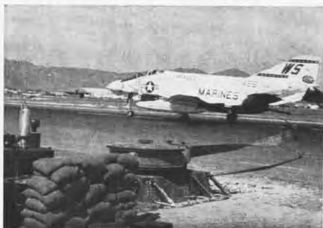
AN F-4B Phantom II of Marine Fighter Attack Squadron 323 is first plane to engage newly installed arrested landing gear at Da Nang.
