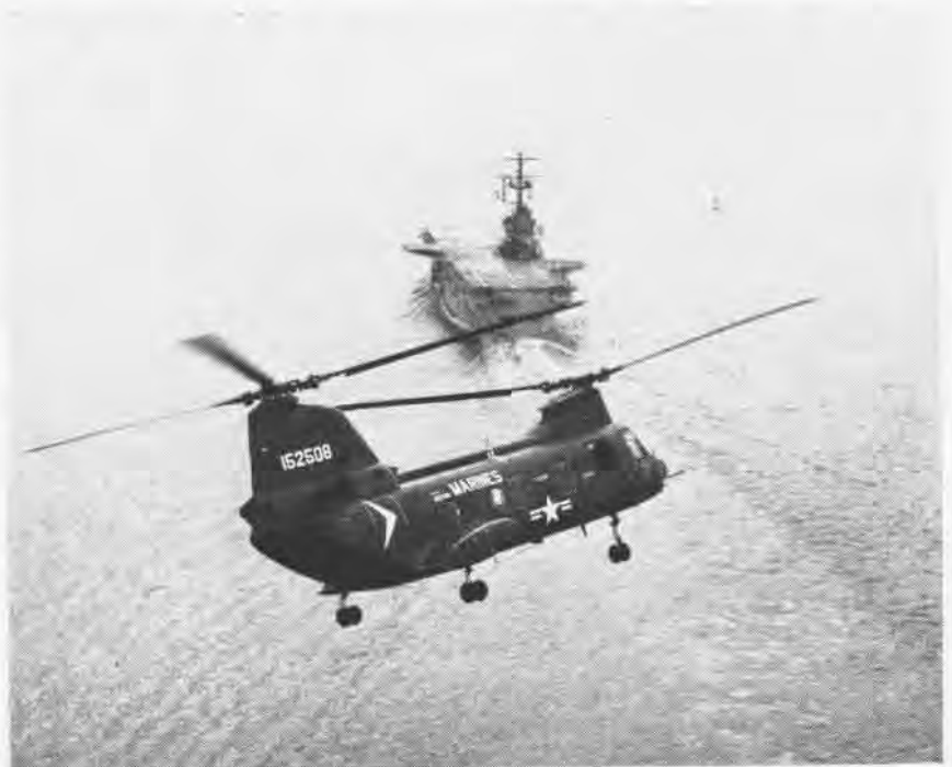
THE BOEING UH/CH-46D Sea Knight medium helicopter has joined the Fleet after completing successfully its Board of Inspection and Survey trials at Patuxent River, Md. It is shown above during its BIS trials; the LPH is the USS Guadalcanal . The "D" model is an advanced version of the -46A Sea Knight now used in Vietnam. More powerful GE T-58-10 turbine engines and "droop snoop" rotor blades are among its new features. These two additions increase its speed and lifting capability. The first -46D's have been delivered to the Marines; the Navy version will be coming off the line later.
