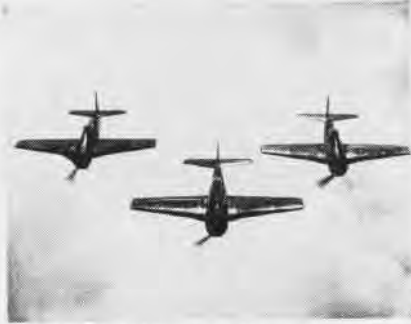
F8F STILL holds record for receipts in standing start to 10,000 feet in 92 seconds.
