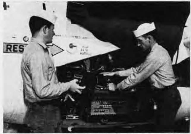
1212: Trouble-shooter Phillips, AE1 (R), determines why Tacan failed, replaces "black box" with one taken from stock in van.
