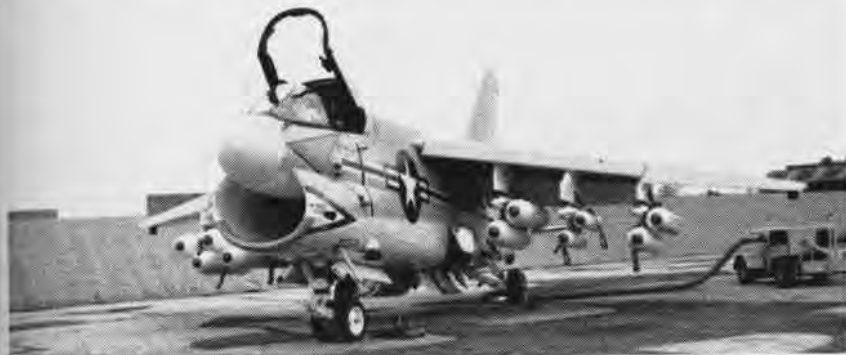
ONE OF NAVY'S newest planes, the A-7A Corsair II, undergoes preflight procedures at the Naval Air Test Center, Patuxent River, Md. Designed for attack and close air support roles, it is being tested at the center for approximately six months. It carries twice the load of bombs of current light bombers, a multiplicity of weapons stores, cockpit armor, self-sealing fuel tanks in critical areas and defense capabilities which include 20mm. rapid-firing cannon and air-to-air missiles. It features not only great ease of maintenance, but also excellent fuel economy. The A-7A can be either land or carrier-based.
