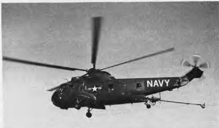
NATC PATUXENT River, Md., is testing a helicopter, manufactured by Sikorsky Aircraft, that has the capability of streaming, towing and recovering mechanical minesweeping gear (described in "Helicopter Undertakes a New Role," NANews , August 1960, pp. 20-24). The aircraft, redesignated the RH-3A, is a modification of the SH-3A. The Naval Air Mine Defense Development Unit, Panama City, Fla., will use the aircraft in its development program of various other mine defenses. In addition to minesweeping gear, the aircraft could tow heavy loads, including small ships, with a force up to 8,000 pounds.
