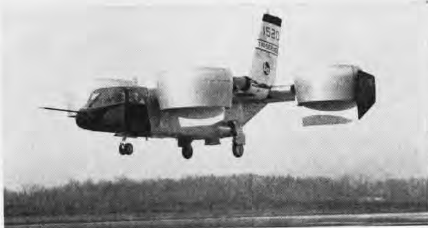
THE TRI-SERVICE X-22A vertical/short takeoff and landing airplane has been flown by Bell test pilots Stanley J. Kakol and Paul Miller, Jr., at Niagara Falls, N.Y. A report stated that the dual-tandem, ducted-propeller craft "handled beautifully, responding to all commands." Textron's Bell Aerosystems Company, which designed and built the VTOL, put the four-engine X-22A through its paces in four takeoffs and landings with its ducted propellers in the vertical thrust position. The X-22A will be tested at NAS Patuxent River.
