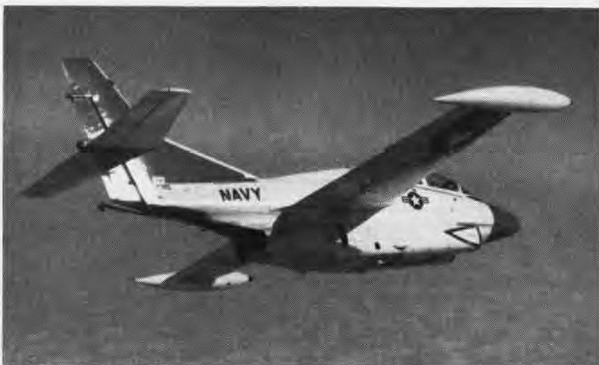
THE SERVICE TEST Division at the Naval Air Test Center, Patuxent River, Md., recently completed the Board of Inspection and Survey Service Suitability Trials of the T-28 Buckeye airplane. This is a twin-engine version of the trainer now used for flight training at NAS Pensacola. One airplane was flown 405 flight hours for twelve weeks on missions which simulated its specified use in the Naval Air Basic Training Command's jet program.
