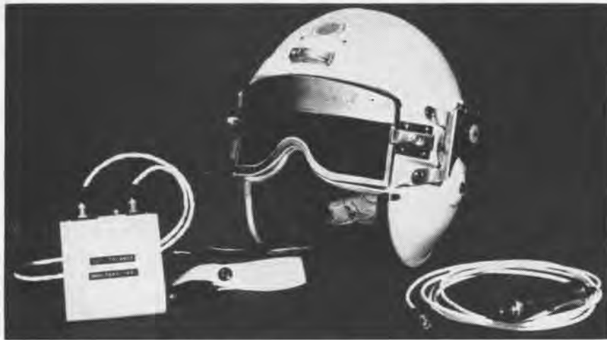
A REQUIREMENT for helmets that was probably unbelievable 50 years ago is shown in the APH-5 modified with a visor to protect the pilot from intense visible radiation.
