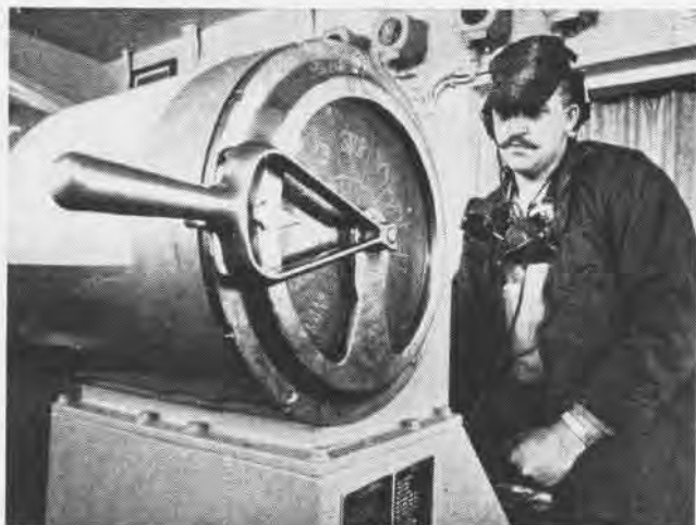
FROM BRIDGE of USS Ranger, G. E. Morrison, SN, can relay C.O.'s speed changes to Engine Room by using the Engine Order Telegraph.
