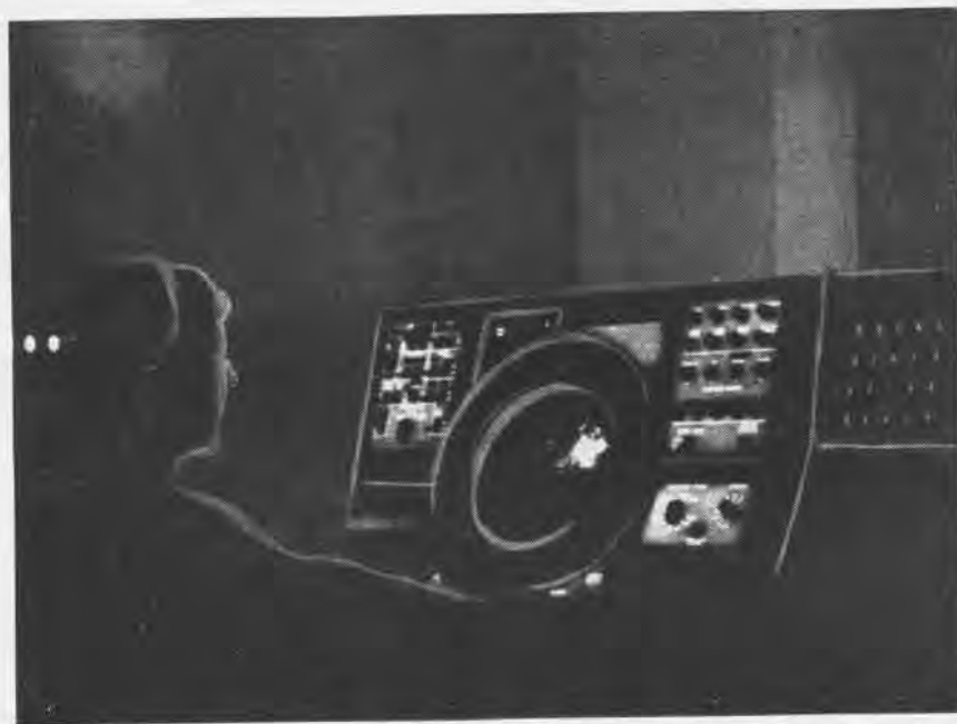
CHRISTMAS TREE is the nickname given to the Fleet Air Control and Surveillance Facility's brightly-lit radar surveillance consoles. They operate on a round-the-clock basis.
