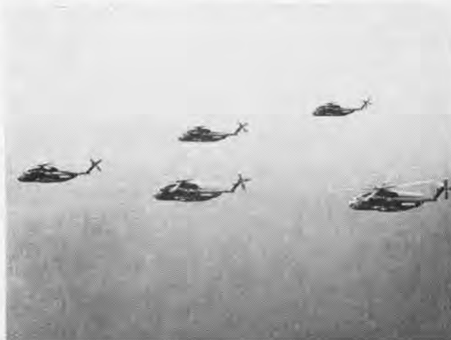
HMH-463, first squadron to get the CH-53A, flew the copters from the East Coast to MCAS Santa Ana, Calif. Formation at right is over Long Island Sound. The CH-53A carries a three-man crew and 38 combat troops or four medical attendants and 24 litter patients. Powered by two turbine engines, it can fly at over 200 miles per hour.
