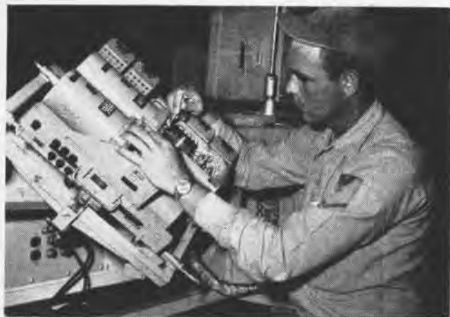
REPAIR of an air data computer is handled by AE2 Gene Gregonis. The component furnishes an F-4 pilot with valuable information.
