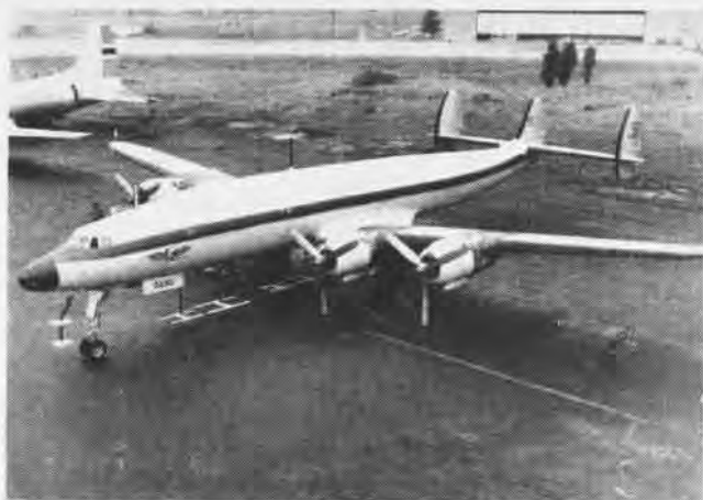
THIS MODIFIED Lockheed Super Constellation, bound for Vietnam, is an advanced version of two similar aircraft known as 'Blue Eagles.' They have been broadcasting TV and radio programs to personnel in South Vietnam since January (NANews, June, p. 24). Unusual antenna arrays are visible atop and below fuselage. The new airborne
