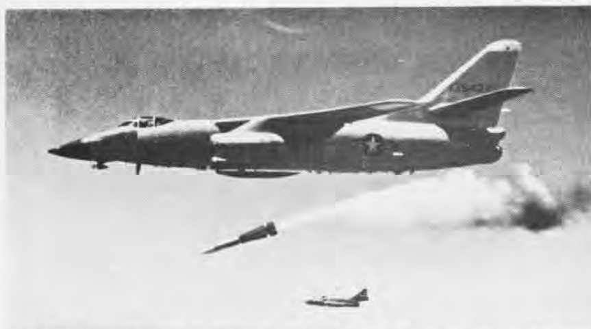
THE FIRST full-scale test of Navy's Phoenix missile and its advanced electronic system took place September 8 over the Pacific Missile Range. An A-3A equipped with Phoenix and its control system located a jet target drone on radar, locked on at long range, and intercepted it in flight. Phoenix is being developed by Hughes Aircraft Co. for use on the F-111B. In photo, taken during earlier test, missile drops from an A-3A Skywarrior.
