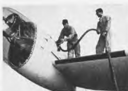
NAS LosAl reservists refuel the 350-gallon wing tip tank of squadron's P-2E.
