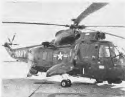
HATS helo showing towed MAD equipment, radar and sonobuoy antennas.
