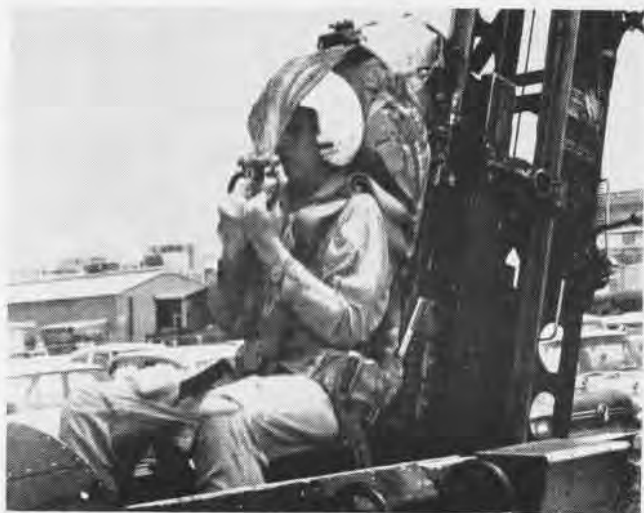
GOING UP in a hurry, Cooper pulls the protective face curtain and starts a swift ride in an ejection seat trainer for jet aircraft.
