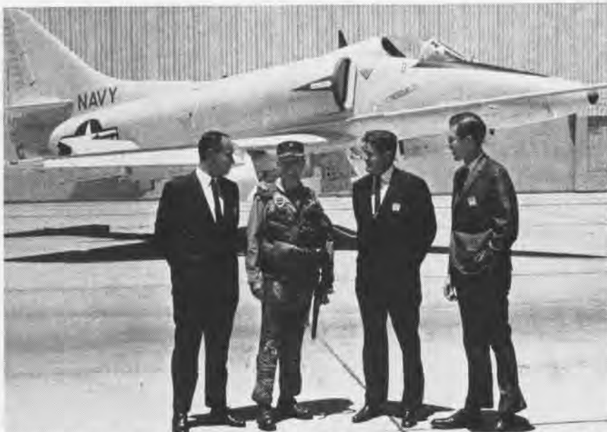
FLIGHT TESTS of the new Douglas A-4F Skyhawk attack bomber began in September. The A-4F features a Pratt & Whitney engine, providing 9,300 pounds of thrust, 800 more than the engine in the A-4E. The new Skyhawk also has steerable nose gear, wing lift spoilers, a zero-zero escape system and updated electronic gear. In front of the Skyhawk are W. E. McKee, Douglas A-4 deputy manager, Cdr. Jack A. Endacott, VA-125 C.O., NAS Lemoore; R. F. Canaday, Douglas Aircraft division director, and J. P. Robinson, a Douglas plant manager.
