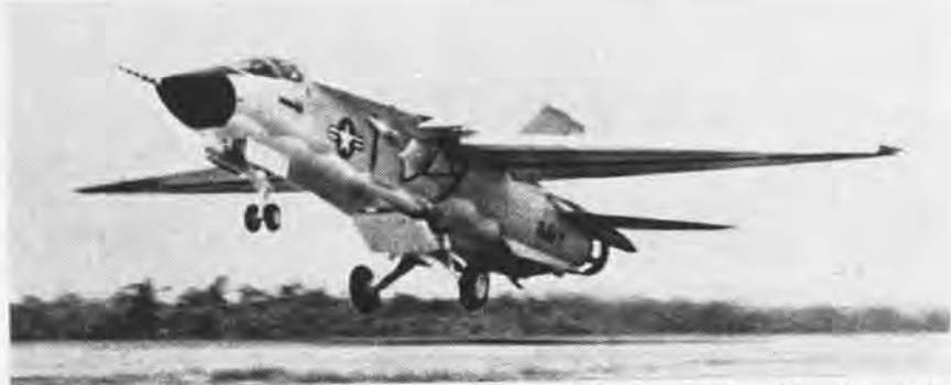
FOUR TRAINING versions of the Navy's Phoenix air-to-air missile, which will arm the Navy F-111B air superiority fighter, are mounted on this General Dynamics/U. S. Air Force F-111A which is being used for weapons separation tests at Eglin AFB, Florida. Two inboard pylons under each wing swivel to keep weapons parallel to the airplane airstream as its wings are swept. F-111's have flown at supersonic speeds close to sea level and at more than twice the speed of sound (Mach 2.3) at high altitudes. The wing-sweep is variable from 16° to 72.5° to provide this wide performance spectrum.
