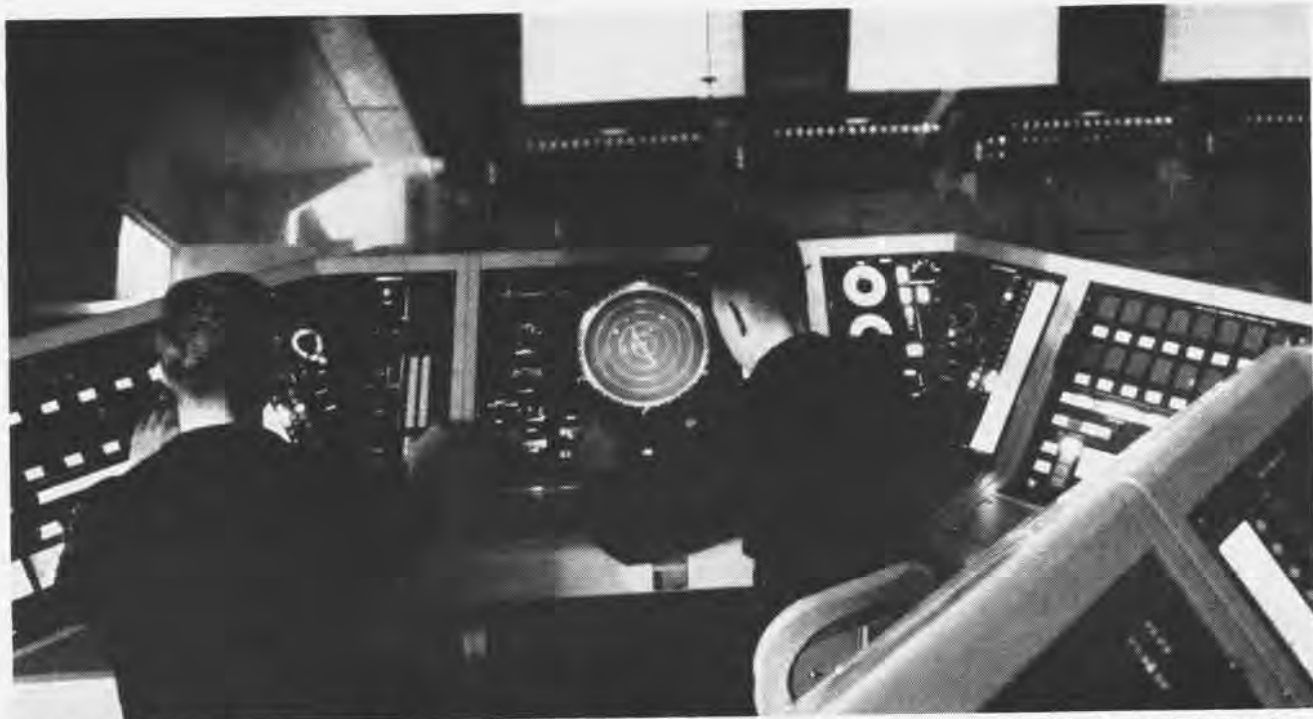
TWO OF FIVE instructors' consoles like those used to control the Trainer are manned by naval personnel. In the background are Pacific Fleet ASW School's 14A6A Coordinated ASW Tactical three display screens which show the progress of an exercise.
