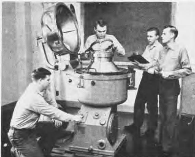
BAYONNE STUDENTS STUDY CENTRIFUGAL PURIFIER SAFETY FEATURE: MOTORS ARE SEPARATE FROM PUMPS
