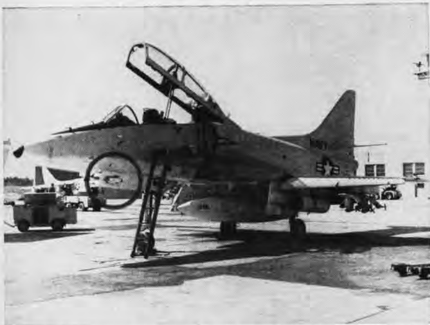
CAMERA (CIRCLE) RECORDS TA-4F'S BOMB RELEASES AND ROCKET FIRINGS
