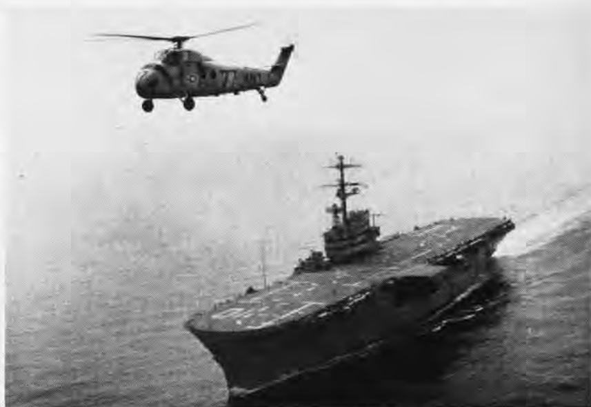
TWO HELICOPTERS , four pilots and two crewmen made up the team from Helicopter Training Squadron Eight, Ellyson Field, Fla., which spent three days assisting the Ingalls Shipbuilding Corporation in calibrating radar equipment aboard USS Tripoli (LPH-10). Ingalls is readying the ship for Navy acceptance later this year. The helicopters flew in the vicinity of Tripoli as technicians tracked them with the ship's radar equipment. Tripoli was commissioned Aug. 6 at Philadelphia with Capt. Henry Suerstedt taking command.
