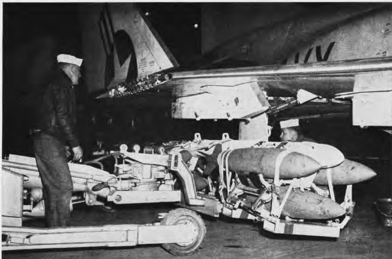
WAHL, AO1, AND SQUIER, AO3, USE SHIPBOARD LOADER TO PUT SIX BOMBS SIMULTANEOUSLY ON PHANTOM II
