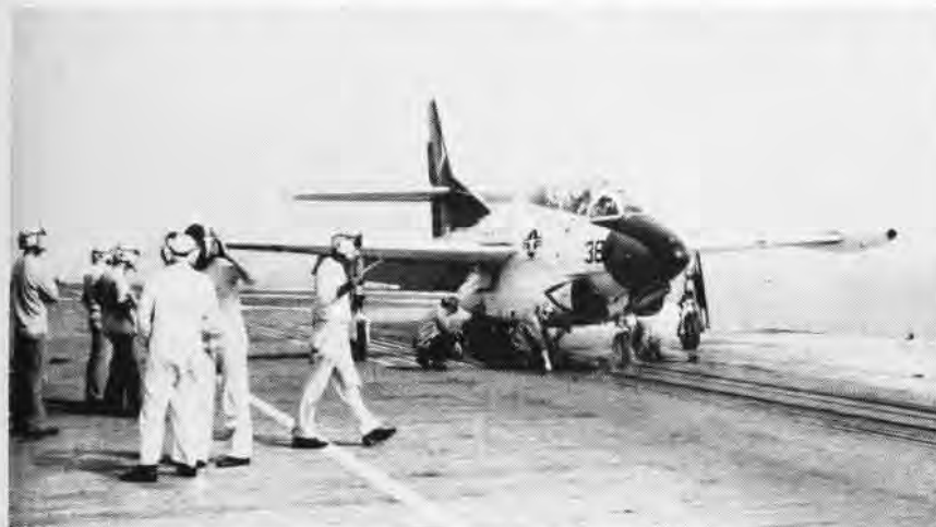
NATTC conducted carrier suitability tests on Lex for the Douglas TA-4F and North American T-28 jet trainers (only T-28 shown) in June. The trainers were tested for service and carrier suitability, flying qualities, and armament and electronics capabilities. The Douglas TA-4F will provide a two-place trainer in a tactical aircraft. This jet is now being phased into the Navy's Combat Readiness Air Wings. North American's T-28 has two J60-P-6 engines rated at
