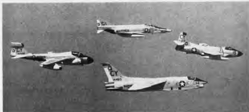
FOUR PLANE COMMAND —Marine Composite Reconnaissance Squadron Two, MAW-2, Cherry Point, used these four jets to surpass the flight safety record for Marine reconnaissance squadrons. The unit's FY 1966 total of 7,614 accident-free flight hours was flown in these aircraft (clockwise, from top): The RF-4B Photo Phantom, EF-108 Skyknight, RF-8A Crusader and EA-6A Intruder. The Phantom will soon replace the older Crusader as the primary photo-recon aircraft for VMCJ-2. The Skyknight and Intruder are designed for active and passive electronic warfare. (Photo by 1st Lt. C. H. Armstrong, USMC.)
