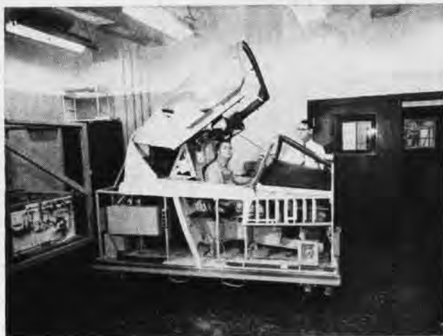
EJECTION SEAT , canopy and radiation shield are used to train maintenance men in operation of seat, how to open and close canopy.
