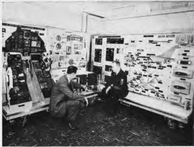
ELECTRICAL SYSTEM unit includes mockup cockpit (left) with switches to activate miniature landing gear, lights, electrical parts.
