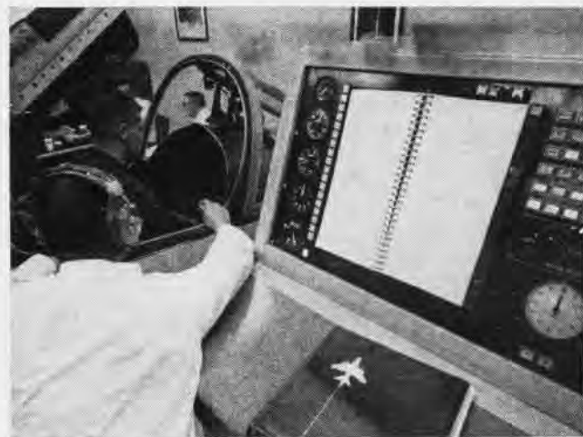
POTENTIAL PILOT gets checkout in the cockpit procedures trainer. The instructor (R) can introduce various emergencies and malfunctions.
