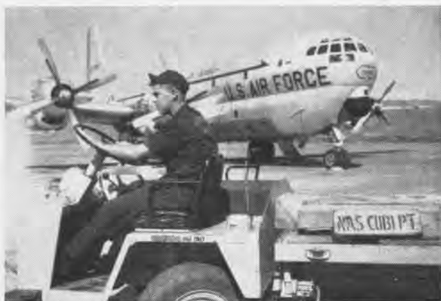
BIG LIFT provided by a hydraulic keylift driven by AM3 Ron Glaus is the major "tool" for loading and unloading transports.
