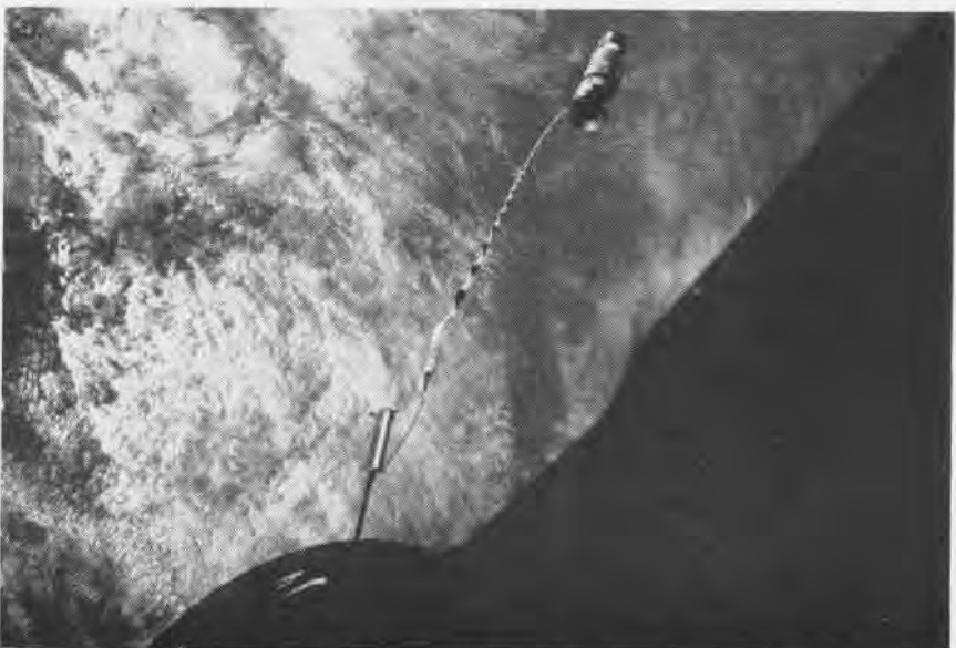
AGENA TARGET docking vehicle orbits the earth, attached to the Gemini 12 spacecraft by a tether Aldrin connected during EVA. Agena was launched 98 minutes before Gemini .
