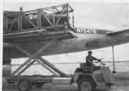
HYDRAULIC keylift brings a drop tank down; operator is ABH2 William W. Moss.
