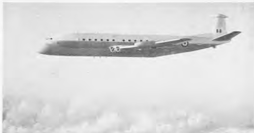
THE FIRST Hawker Siddeley Nimrod, a four-jet maritime reconnaissance aircraft, planned for entry into service with the RAF Coastal Command in the late 1960's, made its first flight from Hawker Siddeley's Broughton airfield on May 23, 1967. The aircraft flew to the company's Woodford airfield where its development program is being carried out. The Nimrod, powered by four Rolls-Royce Spey turbofan engines, is designed to fly at a high subsonic speed and high altitude to the search area, make a low-speed, low-level patrol and a fast return to base.
