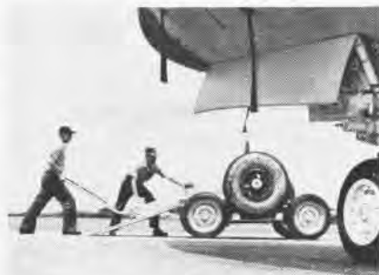
AT NAS Barber's Point, AMH2 Barry L. Fillmore and AMS1 Duane J. Zaleskie use a new tire changer kit built by Fillmore for use with the Orion. It carries two main wheels, two nose wheels, jack and tool box. Two men, using the new emergency kit, can change a blow-out in about one-half hour.
