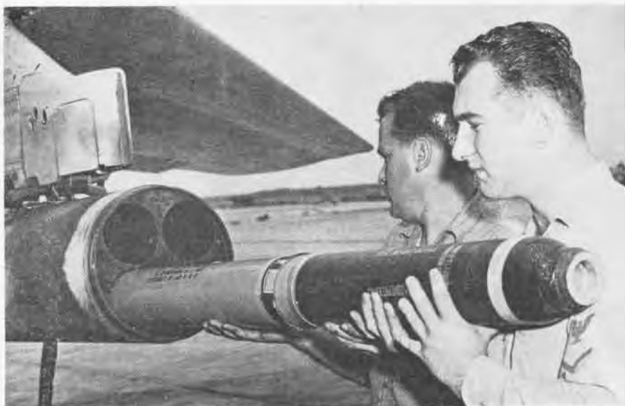
AO3 REDMAN AND AO2 NORMAN LOAD ZUNI ROCKET INTO POD MOUNTED ON CORSAIR II
