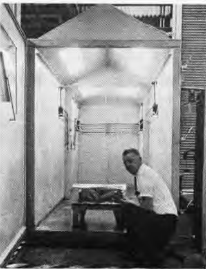
WALKER CHECKS FOR JET PART CORROSION
