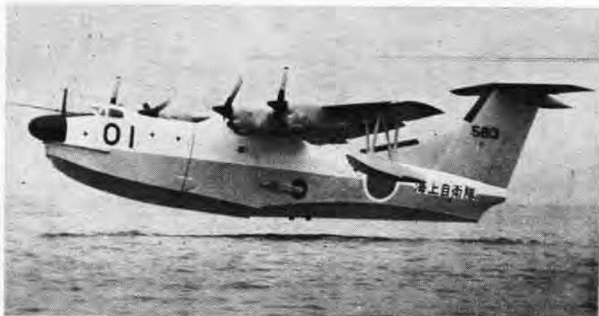
THE FIRST flight tests of the Japanese PX-S STOL flying boat were successfully completed recently. Powered by four T-64 engines, it has a maximum speed of approximately 300 knots, a cruising speed of approximately 200 knots and a maximum cruising range of more than 2,500 miles. The ASW aircraft is designed to take off and land in heavy seas at 45 knots. In addition to carrying the standard ASW detection equipment, the PX-S boasts a dunking sonar capability.
