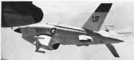
FIREBEE IS LAUNCHED FROM WING OF DP-2E NEPTUNE
