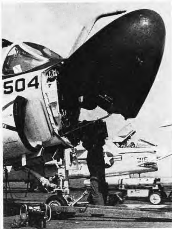
BECAUSE the Intruder's equipment is designed to be interchangeable, it's no trick at all, once the nose is flipped up (above), for this VA-165 technician to remove electronic equipment and quickly replace it. Below, pilots check their ordnance loads. At right, an Intruder taxis in from a landing after completing its mission.
