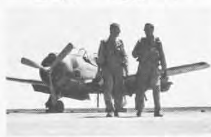
THE T-28 basic propeller trainer, shown above with Navy and Marine Corps students, has performance similar to early WW II fighters. Successful carrier qualifications (below) complete this training phase.
