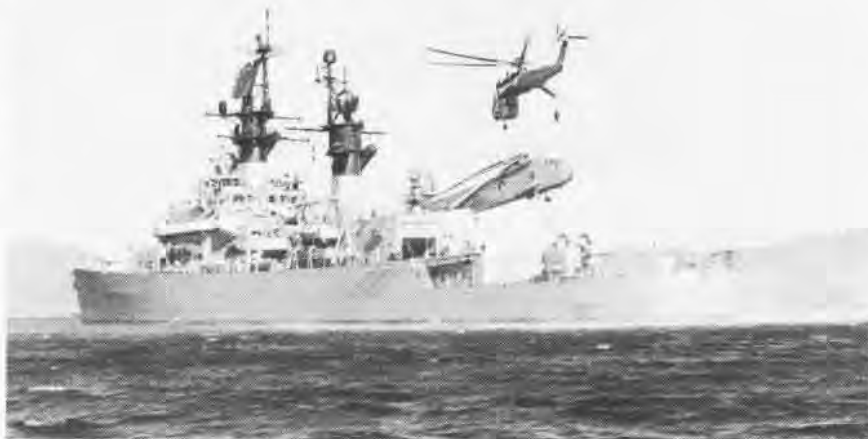
A U.S. ARMY CH-54A Sky Crane lifts a disabled Navy SH-3 Sea King from the deck of guided missile frigate USS Jouett (DLG-29) in the Tonkin Gulf. Navy helos operate from the decks of destroyers to rescue aviators. The Army craft took the helo to a nearby repair facility. Later the SH-3 Sea King returned to its primary mission of search and rescue.
