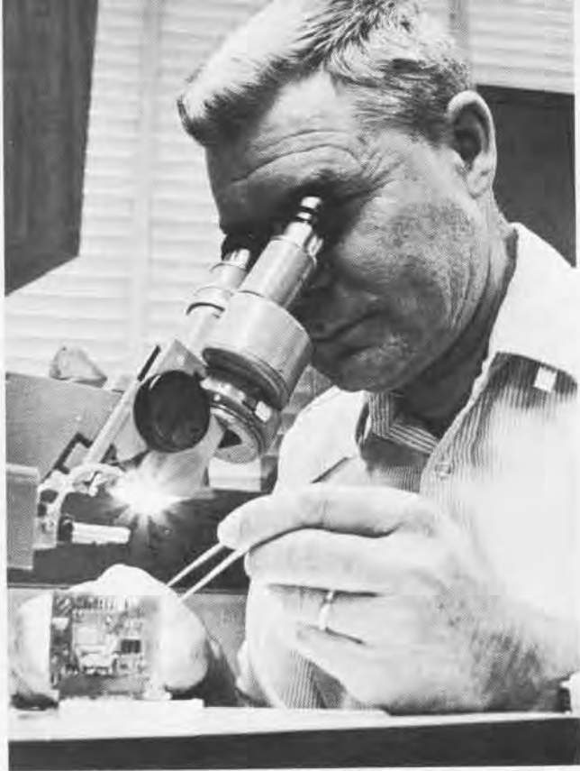
AN ELECTRONIC model maker in Point Mugu's electrical devices section uses tweezers under a ten-power microscope to assemble a miniature circuit board for the airborne television set.
