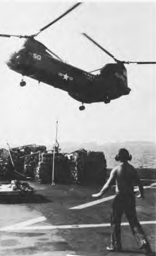
UH-46 from Niagara Falls approaches hook-up pole which is connected to cargo pallets.
