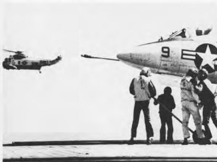
SH-3A SEA KING of HS-80X1, above, stands by as plane guard for aircraft flown from Intrepid . New Orleans-based A-4, right, catches #1 wire.
