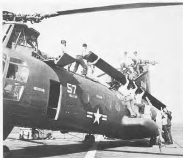
Sea Knight of vertical replenishment detachment aboard supply ship has new rotor blade installed during routine maintenance. Below, SH-3A approaches DLG landing platform at the end of a mission.
