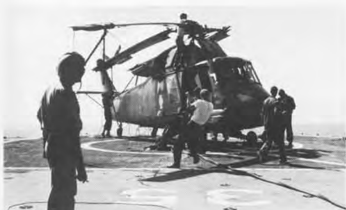
Ground crew manually spreads rotor blades of a Seasprite which is being readied for a flight from DLG operating near the Vietnam coast.
