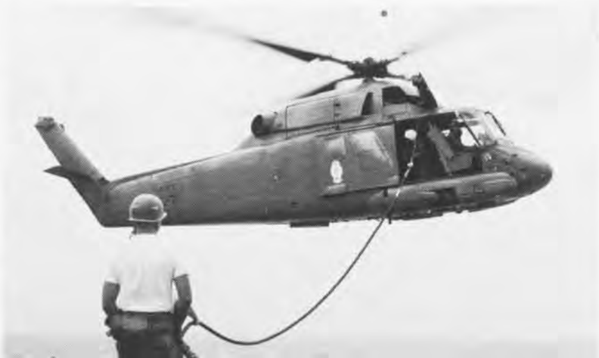
Sixty crewmen and maintenance personnel of HC-7's Det. 110 move their personal gear and 18,000 pounds of support equipment each time they change to a new host aircraft carrier. Below, armored Seasprite takes on fuel from the deck of a DLG in the South China Sea.
