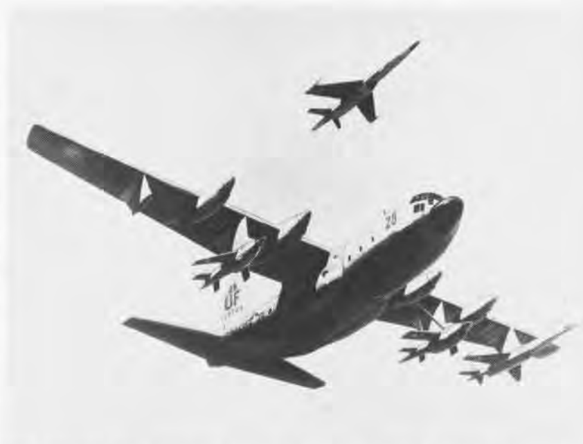
TWO NEW DC-130A launch and control platforms for target drones will be delivered to NAS North Island's VC-3 in August. As depicted in the drawing above, the converted C-130's will carry and operate four drones in support of training exercises. Drone launching aircraft, currently in the Navy inventory, accommodate only two target drones per flight.
