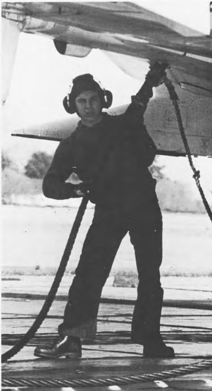
Preparing for launch, a flight deck crewman holds bridle until slack is taken out while, below deck, ABE3 Michael Toco checks the steam pressure, top.
