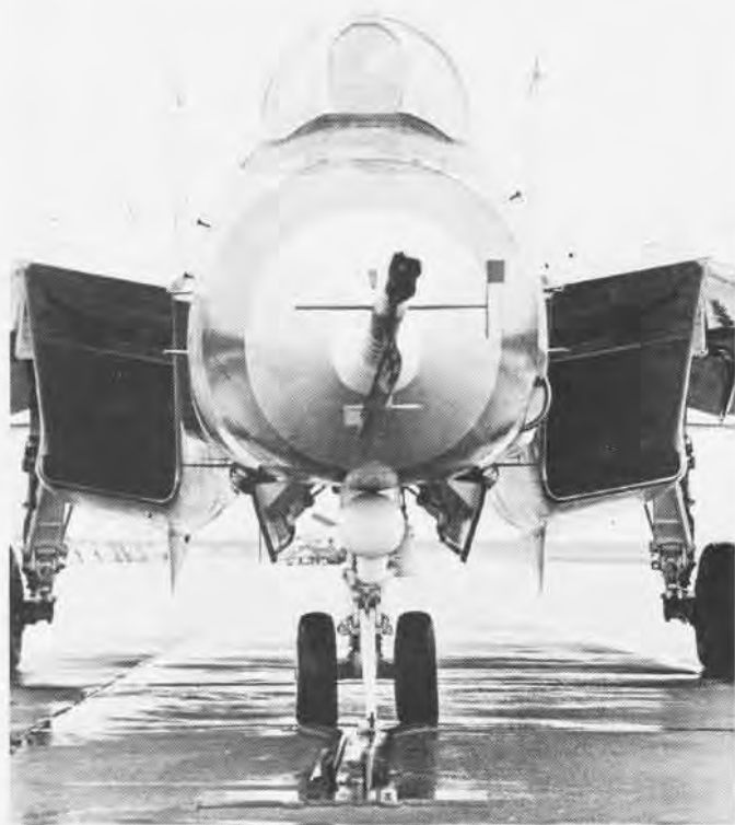
In catapult spotting tests made by the Tomcat evaluation team, the launch bar must slide easily into the nose tow track. Guiding LCdr. Tucker in the F-14 is Lt. Mark Welford.
