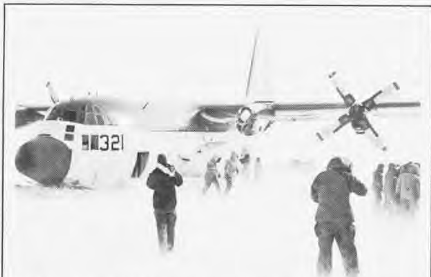
The damage to the LC-130 Hercules was extensive. Note inboard engine and landing gear.
