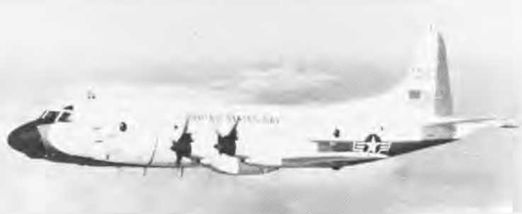
Oceanographic Development Squadron Eight's newest aircraft, an RP-3D, arrived at NATC Patuxent River in November. The Project Magnet Orion was selected by the Naval Oceanographic Office as its new platform for measuring the direction and intensity of the changes in the earth's magnetic field. Navy has pioneered in airborne magnetic surveying since WW II.
