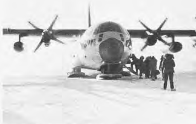
At left, crewmen from VXE-6 attach JATO bottles to the fuselage of an LC-130 Hercules. JATO provides the extra lift needed to get the fully loaded aircraft off the ice and into the sky. After an hour and a half on the ice at Amundsen-Scott South Pole Station (with temperatures at minus 48 degrees), passengers embark aboard LC-130.
