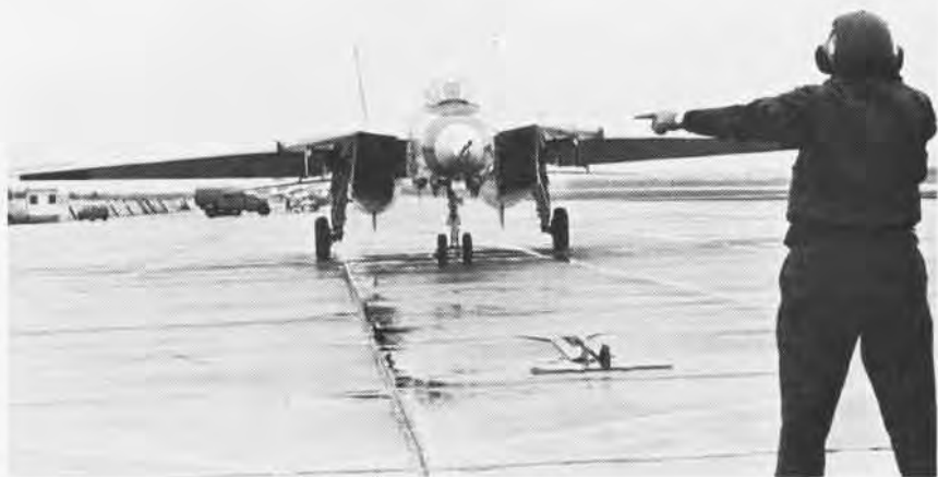
In catapult spotting tests made by the Tomcat evaluation team, the launch bar must slide easily into the nose tow track. Guiding LCdr. Tucker in the F-14 is Lt. Mark Welford.
