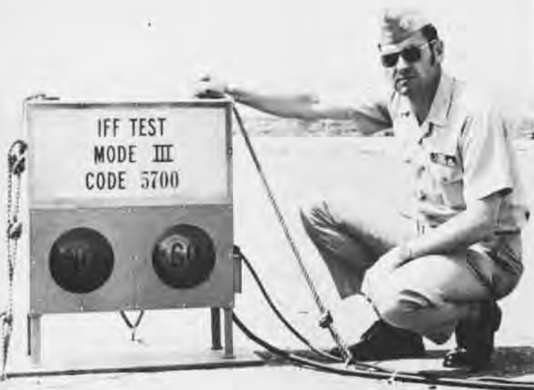
LCdr. W. C. Ellis, NAS North Island, developed the go-no-go system which automatically tests IFF and SIF capabilities of aircraft as they taxi over it on the way to the runway.
