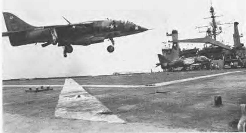
During shipboard operations aboard USS Raleigh (LPD-1) the versatile AV-8A Harrier carrier qualified on still another category of ship and added a new aircraft to the LPD's capability.
