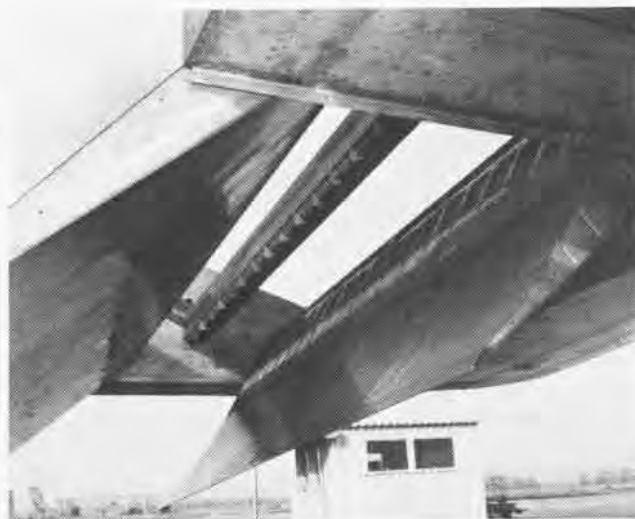
The XFV-12A will be able to carry a varied weapons load, above. At right is a close-up of the augmenter component test fixture which is mounted at the end of the 100-foot rotating arm, below; the rotary test device is being used to verify thrust augmenter parts. The illustrations opposite show the A-4 Skyhawk and F-4 Phantom II assets going into the XFV-12A, top; engine airflow through the ejector system, center; and the airflow through the engine in horizontal and vertical modes, bottom.
