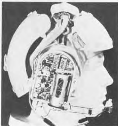
What's inside? The three-pound helmet for flight deck personnel, left, incorporates a transmitter in the right ear pad and receiving equipment in the left pad, center. Photo at right confirms that "through the ages, the helmet had great esthetic value."
