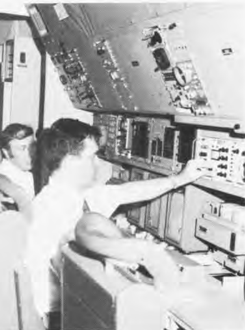
Dr. Weiffenbach, top (left), and Dr. Guler are on the Johns Hopkins satellite team with Robert L. Hickerson, above (foreground), who adjusts Omega navigation and display panels and controls for automated geomagnetic airborne survey system aboard the RP-3D.
