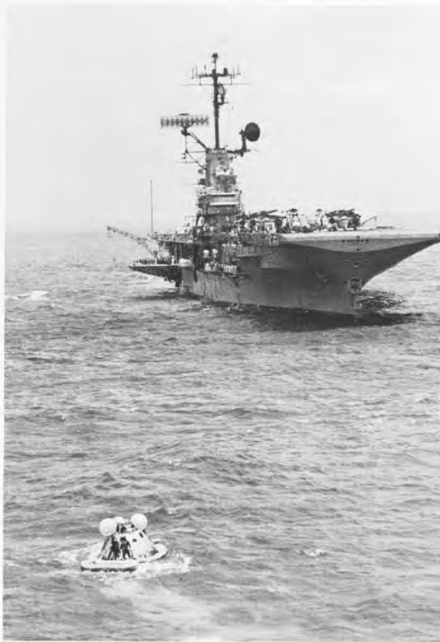
System satellites, tracking stations and ship receivers put USS Hornet on target to recover Apollo 12 command module. With the navigation satellite set, Hornet was only 3 1/2 miles from the splashdown point.
