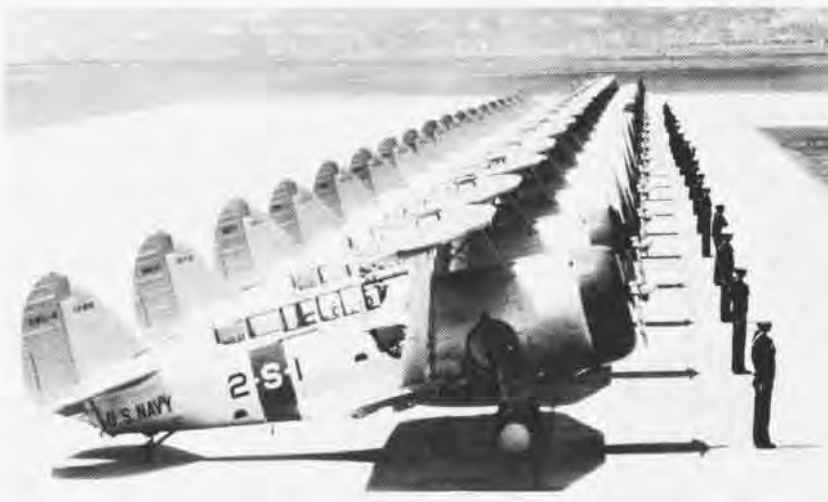
SBC-4s, last carrier biplane dive bombers to enter service, incorporated other features of new monoplanes that also became operational in the late 30s.
