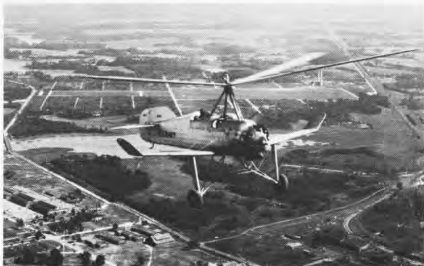
Pitcairn XOP-1 autogiros were civilian models procured for Navy and Marine evaluation of new concept. Rotor was turned by airflow rather than power.
