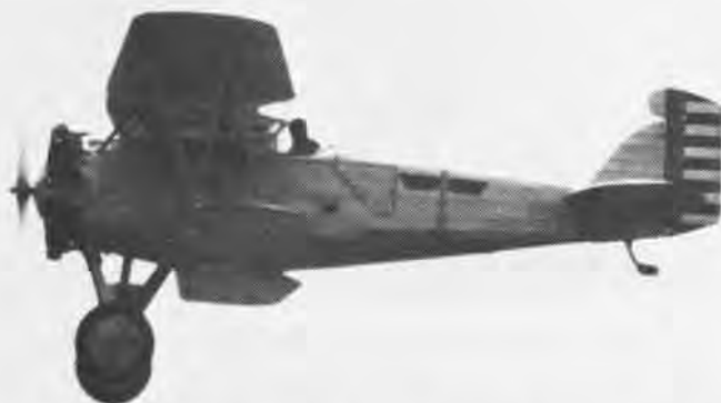
Boeing XF3B-1, one of several prototype fighters designed to use P&W Wasp, was tested in 1927 for either carrier or, equipped with floats, battleship ops.
