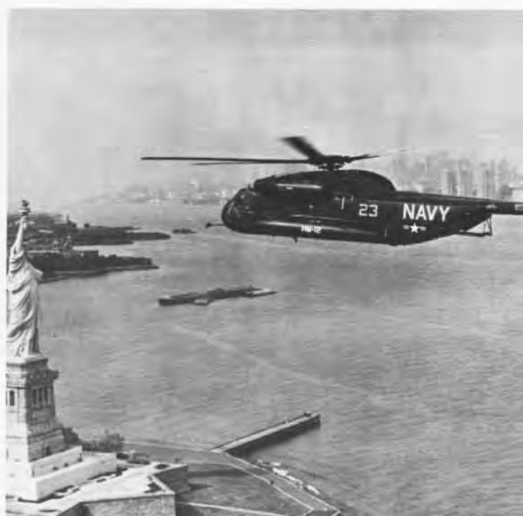
Sikorsky RH-53Ds are specially equipped Sea Stallions used for mine countermeasures service, towing various sweeping gear.
