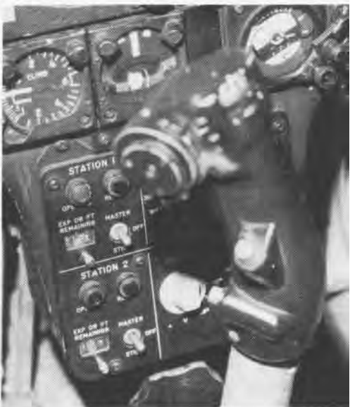
KS-87B camera is newest type used in Crusaders . Close inspection of cockpit gauges below, shows special photo panel by stations.
