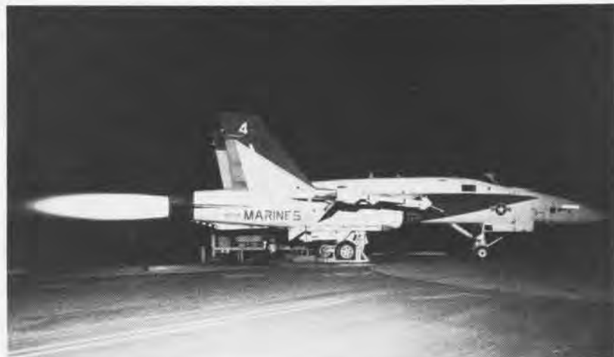
F/A-18 night high-power run test.
