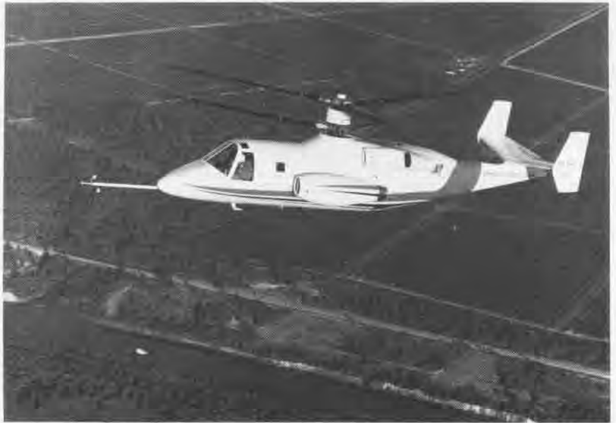
The XH-59A ABC demonstrator was designed and built by United Technologies' Sikorsky Aircraft to evaluate the feasibility of the ABC rotor system through flight testing as a pure helicopter, and at high speed in the auxiliary propulsion mode using side-mounted jet engines.
