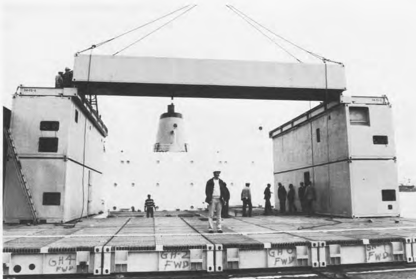
ARAPAHO modules feature aluminum roller-curtain hangar bay doors, maintenance shops, power generators, spare parts stowage, ready rooms, and a magazine sufficient to support a deploying helicopter detachment.
