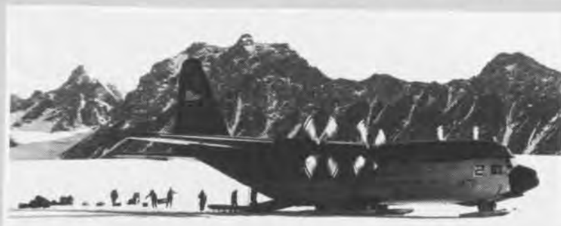
A ski-shod Lockheed LC-130 Hercules transport offloads at a field camp in the Morozumi Mountain Range, Antarctica.
