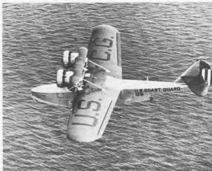
This Douglas RD Dolphin was the second of 13 of these amphibious aircraft built for the Coast Guard in the early 1930s and used in search and rescue operations.
