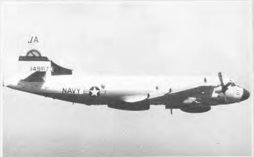
VX-1's EP-3A outfitted with EMPASS gear.
