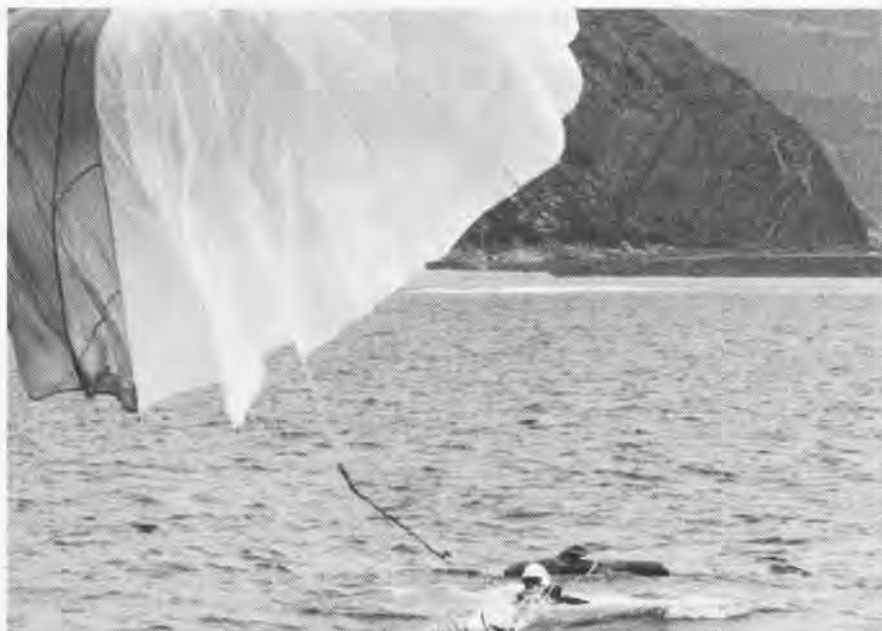
During one of many tests, the pilot is freed from his parachute immediately as the Seawars device automatically releases his Koch fitting upon immersion in salt water.
