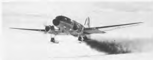
A VX-6 R4D taking off from Byrd Station, Antarctica, using JATO rocket boosts, in December 1962.
