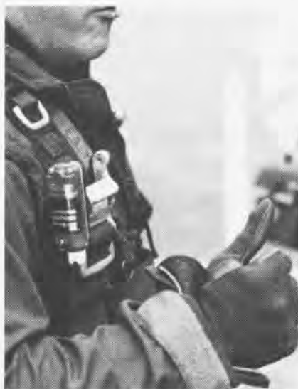
Mounted on the Koch fitting, the Seawars device is designed to not interfere with manual release procedures.
