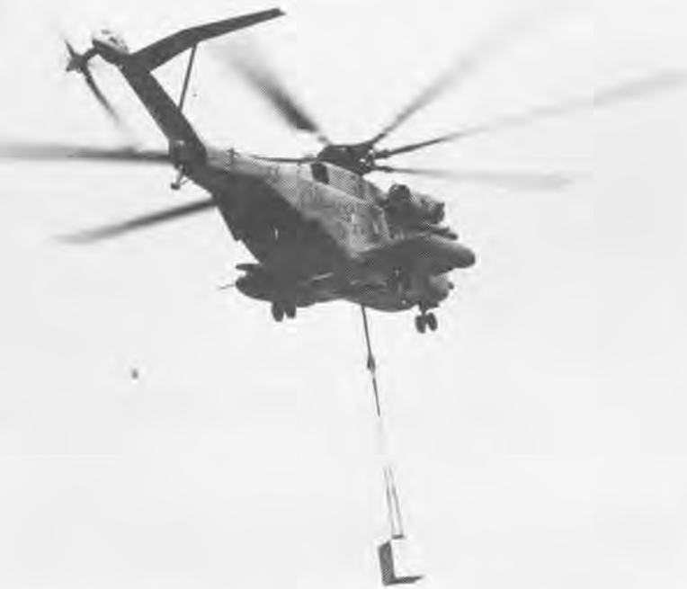
A CH-53E Super Stallion, seen here carrying a 16-ton cement block at MCAS(H) New River, S.C., can lift far more weight than any other type of Marine helicopter.
