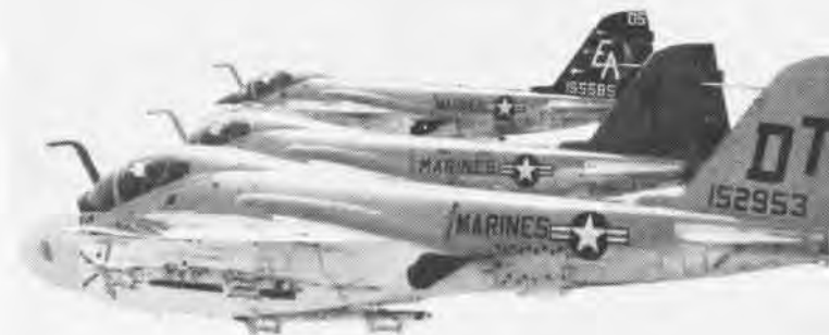
The A-6 Intruder is an all-weather attack aircraft capable of delivering up to 15,000 pounds of ordnance with pinpoint accuracy.
