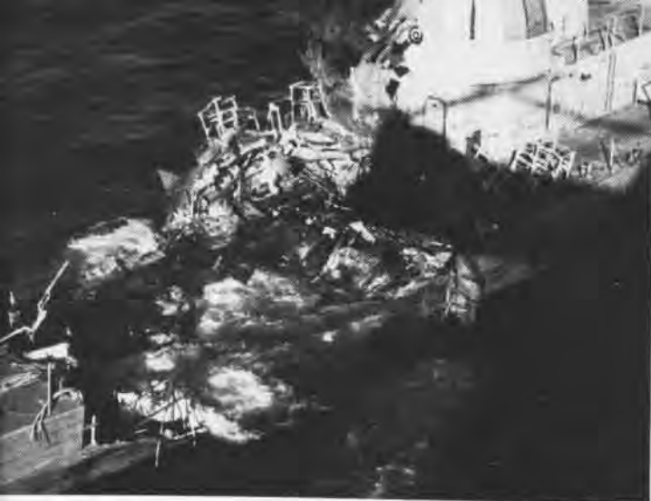
A devastated bow section of a target destroyer attests to the power packed by the Harpoon missile.
