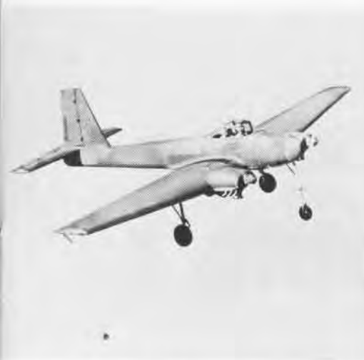
Above, the TDR-1 was used by the Navy's Special Air Unit One as a remotely-controlled training drone during the early 1940s. Below, pilotless, explosive-laden PB4Y-1s like this one over Bay of Biscay in 1943 were used operationally in attempts to hit enemy targets.
