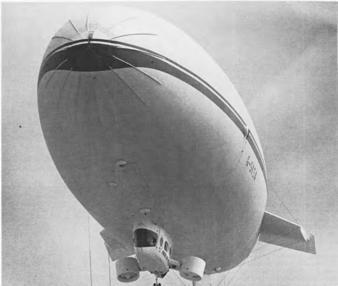
The remarkably agile, British-built AI-500 blimp, with its unique vectored-thrust propulsion, was demonstrated at Andrews Air Force Base near Washington, D.C., during the spring of 1983.
