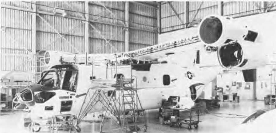
Top, an artist's conception of the V-22's cockpit with the Osprey in nighttime operations at sea. Above, the second of six Ospreys being built for the V-22 development program is seen in final assembly at Bell. After initial flights there, it is scheduled for major testing at Boeing's flight test facility in Wilmington, Del.
