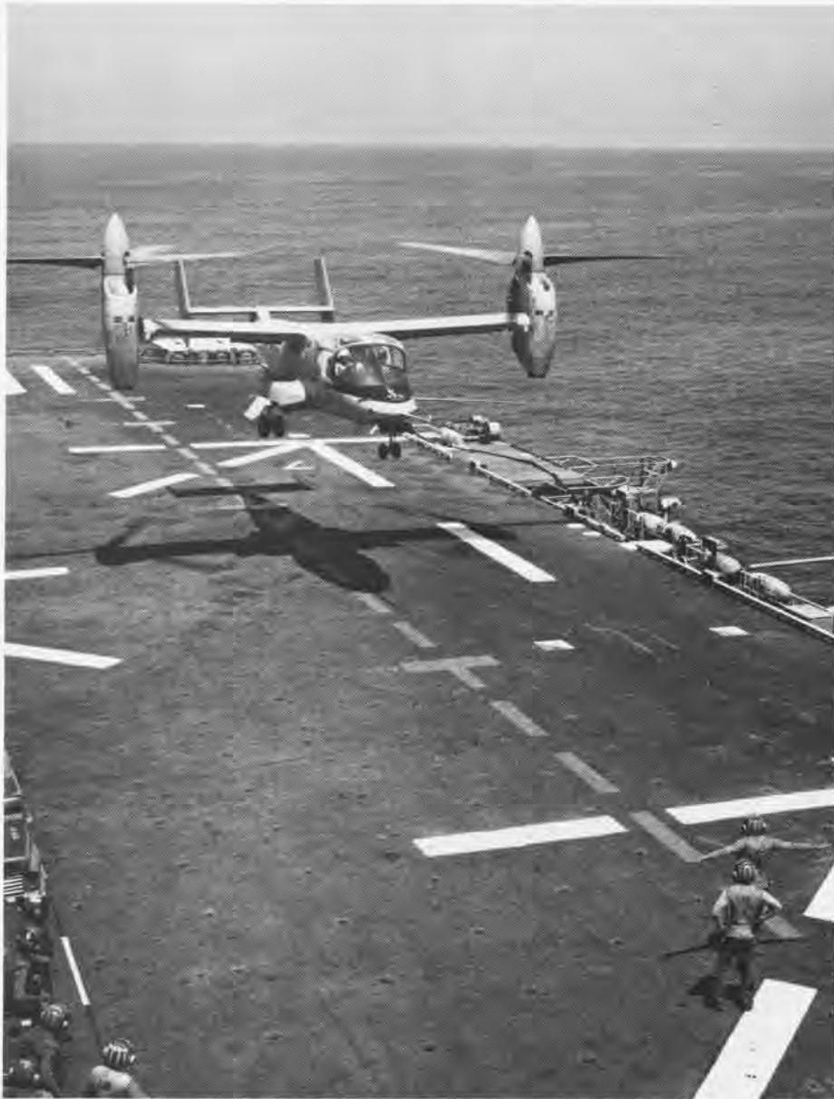
Successful shipboard trials with one of the two Bell XV-15 tilt-rotor research aircraft were conducted on Tripoli (LPH-10) in 1982.
