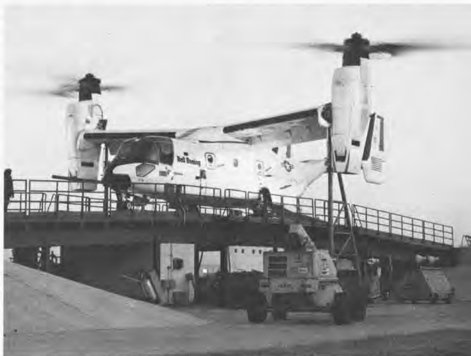
The first V-22 running up on elevated test stand at Bell's Arlington, Texas, flight test center in preparation for first flight. The elevated stand allows operation through full proprotor tilt range.
