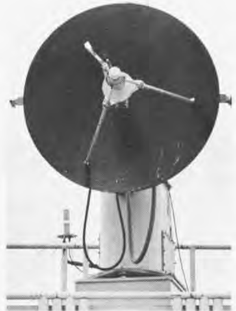
NATC Patuxent River conducts tests with AN/SPN-46 radar that are identical to those aboard a carrier.
