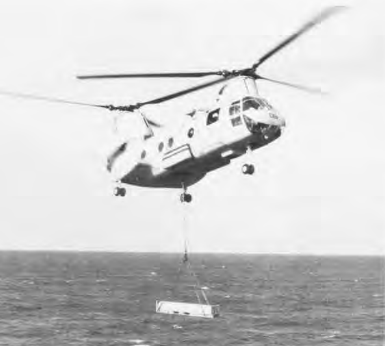
An HH-46D of HC-6 Det 6 carries cargo to Wasp (LHD 1). The 30-year-old Sea Knight—called the workhorse of the fleet—is critical to the Navy's logistics operations.
