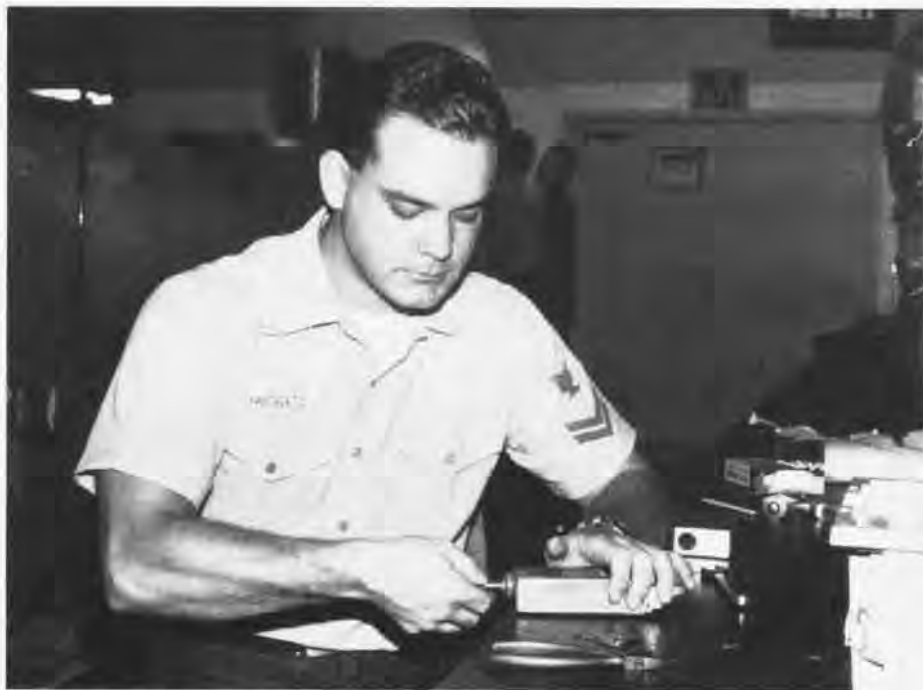
AE2 John D. Roberts, of the AIMD at NAF Washington, D.C., replaces a cracked cover of an actuator for a P-3 auxiliary power unit.
