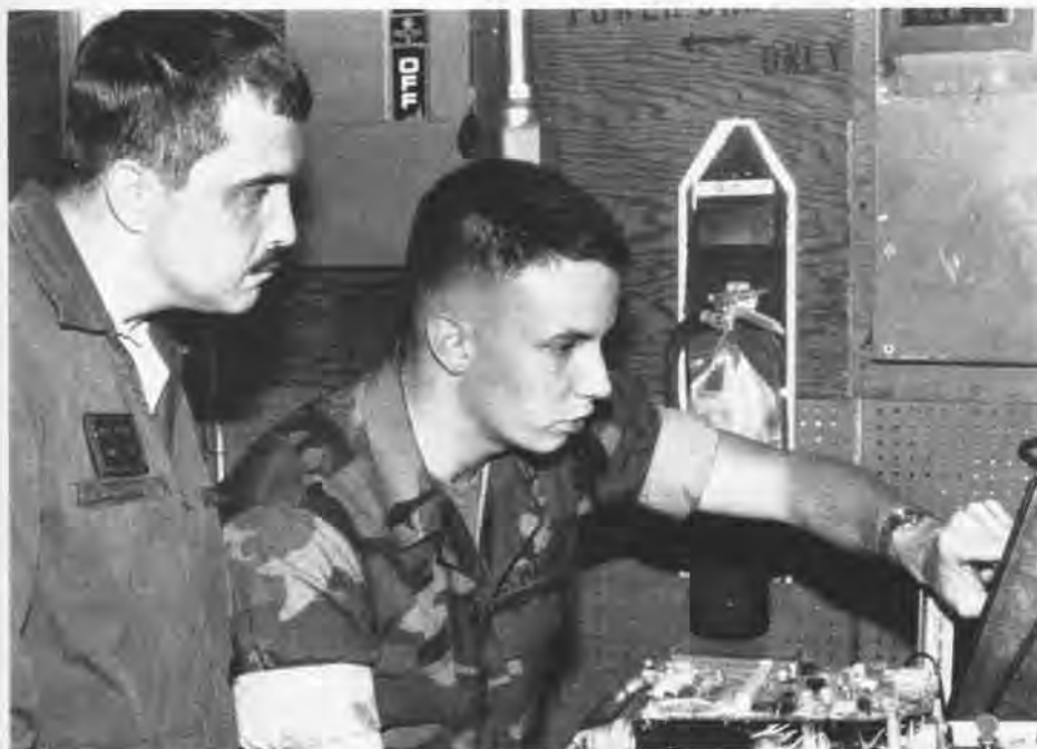
At AIMD, NAF Washington, D.C., Lance Corporal Christian S. Wolf troubleshoots an EA-6B supervisory panel, which maintains voltage coming off the aircraft's generators, while AE2 Mark Olinger observes.
